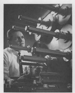
MYLAR STRIP AND METAL FOILS are wound together on this machine to fabricate an electrical capacitor. Lee Amador (4233-2) learned to operate such equipment with a variety of materials, as well as to prepare miniature coils, capacitors, and other components with specialized manipulating devices. Time spent in learning shop techniques was offset by hours of theory study. Lee came to the Electronics Apprenticeship program from Documents organization. He's been at Sandia Laboratory for five years.
